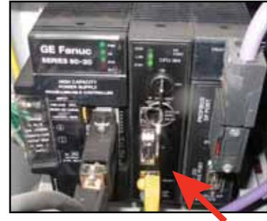
**Figure 3: Press the Release Latch to Remove Card**
